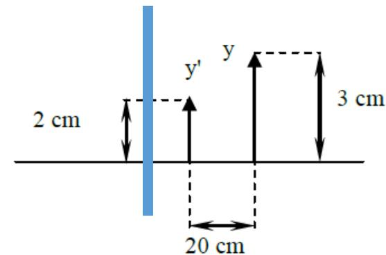
$$\frac{1}{x_o} - \frac{1}{x_i} = \frac{1}{f_o} \quad f_o = \frac{n_M}{n_L - n_M} \left( \frac{R_1 \cdot R_2}{R_1 - R_2} \right)$$
